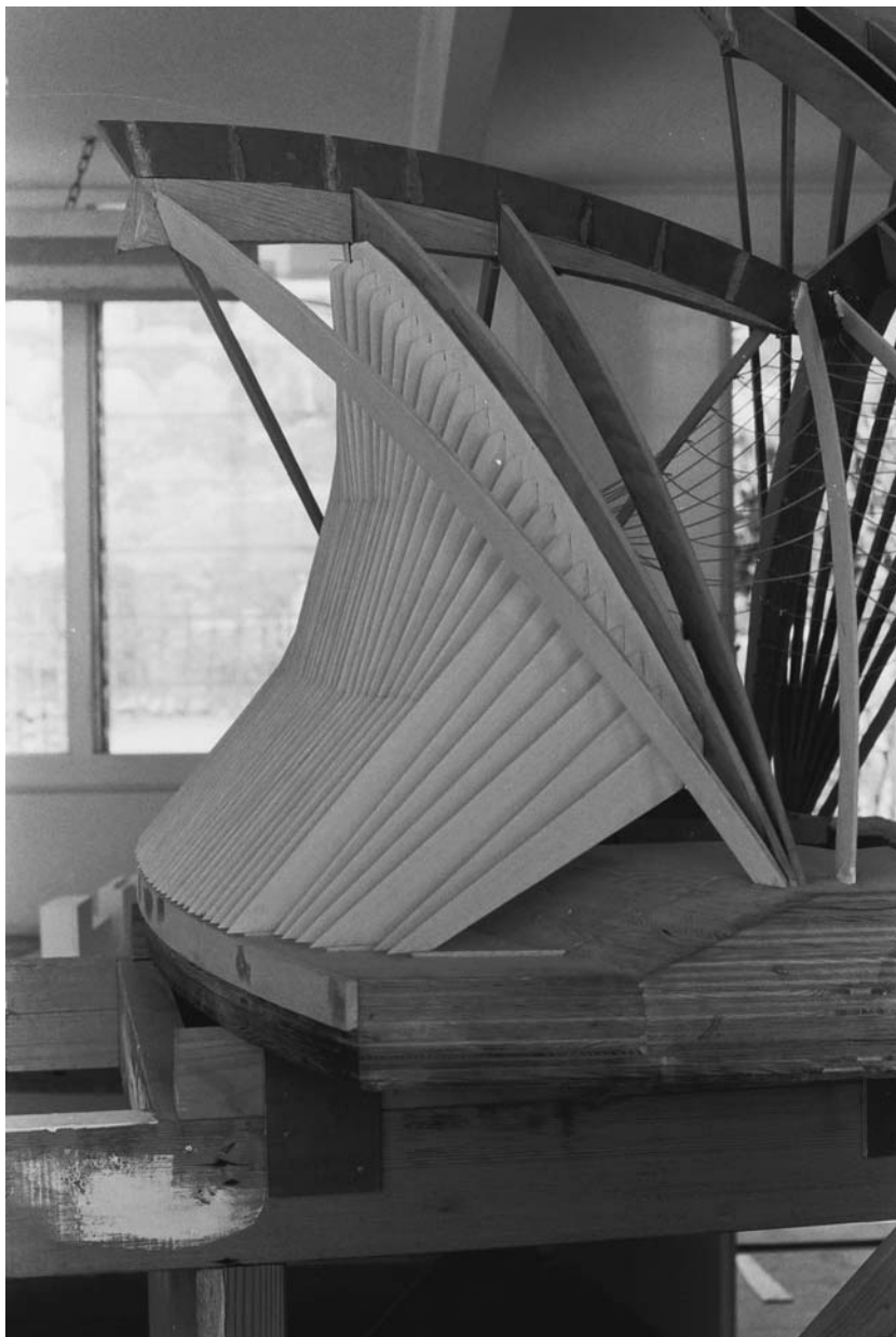
Figure 4: Hall Todd & Littlemore study model of Utzon's last northern glass wall scheme, early 1967.
